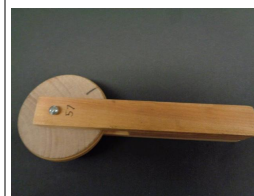
Jerry Johnston's tool for measuring linear feet to scale
