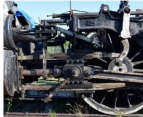
The eccentric rods came free with relatively few hours of work. The left side electric crank came off using mostly "sweat equity," but the right one required placement
