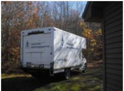
truck needs to be replaced. In order to do that, the body would need to be lifted off the frame. There is a good possibility that lifting the body would break the seal between the body and the cab and create water leakage.
