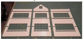
Next these pieces are 'snapped' together prior to gluing to the wooden substructure using Gorilla Super Glue Gel.
