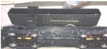
Jamie also presented a simple method for removing lettering from rolling stock. Simply painting over the lettering typically still leaves the lettering visible. To remove the lettering, Jamie purchased a cheap set of scratch brushes from Harbor Freight.
