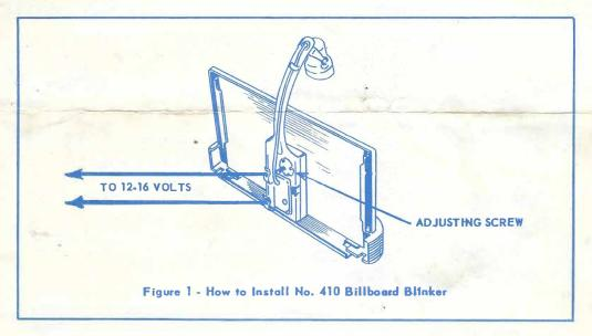
No. 410 Billboard Blinker is made to fit any Lionel billboard sign. The blinker base slides on the frame of the billboard from the back so that the lamp bracket curves over the front of the hillhoard.
